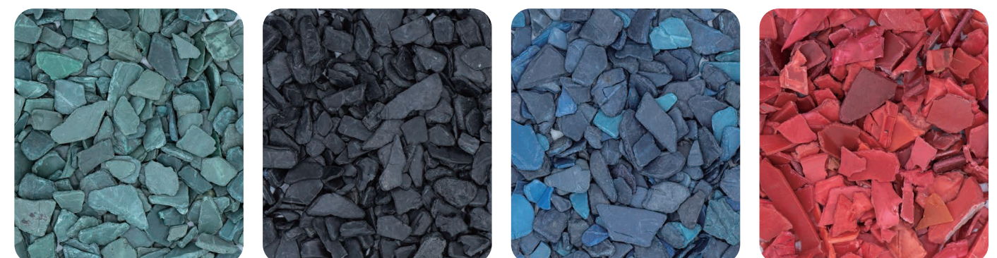
Color & polymer sorting of the plastic shell for daily packages and household appliances
